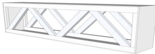
Fig. P.2.3 Wooden frame of truss lintel
